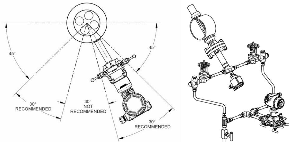
With this installation, the primary element is installed in the pipe with the instrument connection in the lower half of the pipe. From the instrument connections the impulse lines are routed downward towards the transmitter, and the wet legs isolate the transmitter from the heat of the process steam.
