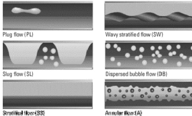
Figure 1: Two-phase flow patterns
