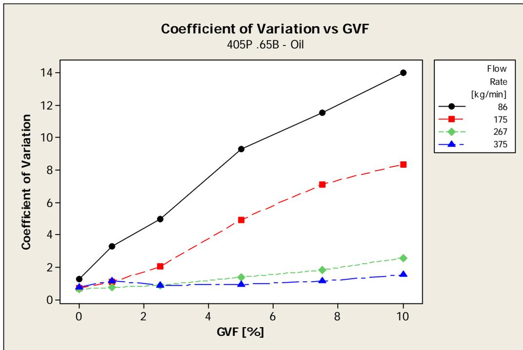
Figure 5: Coefficient of Variation Sensitivities to Varying GVF at Multiple Flow Rates
