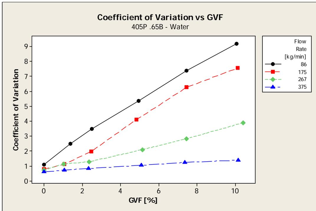
Figure 3: Coefficient of Variation Sensitivities to Varying GVF at Multiple Flow Rates
