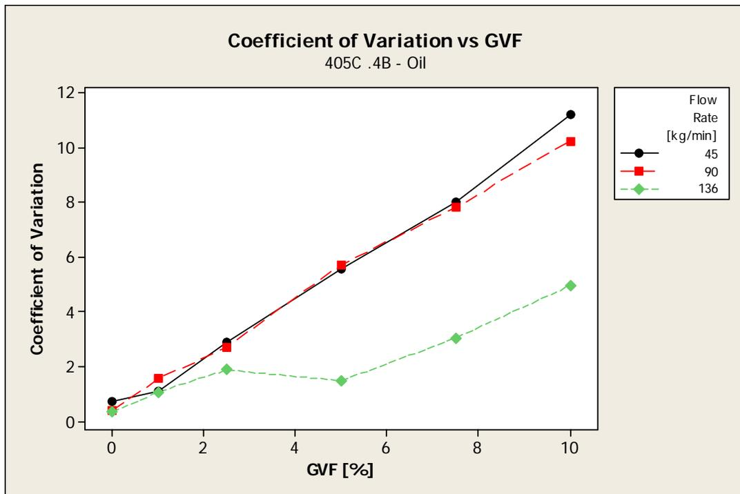
Figure 9: Coefficient of Variation Sensitivities to Varying GVF at Multiple Flow Rates
