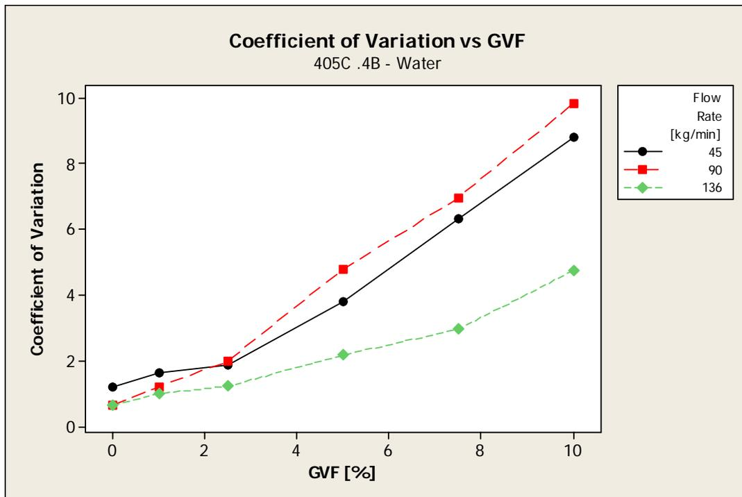
Figure 7: Coefficient of Variation Sensitivities to Varying GVF at Multiple Flow Rates
