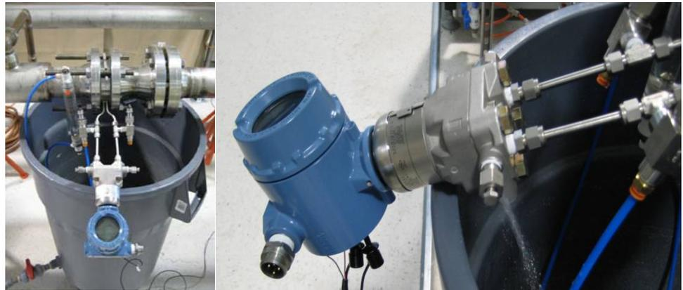
The data represented in Figures 3, 4 and 6 were taken while the pump was running at 1850 RPM. This generated an initial DP of approximately 50 inH<sub>2</sub>O across a 0.45 $\beta$  orifice plate with a corresponding standard deviation value of 0.18 inH<sub>2</sub>O. Once flow conditions had stabilized, a 0.35 gallon per minute leak was created on the low side impulse line. Immediately, the standard deviation
