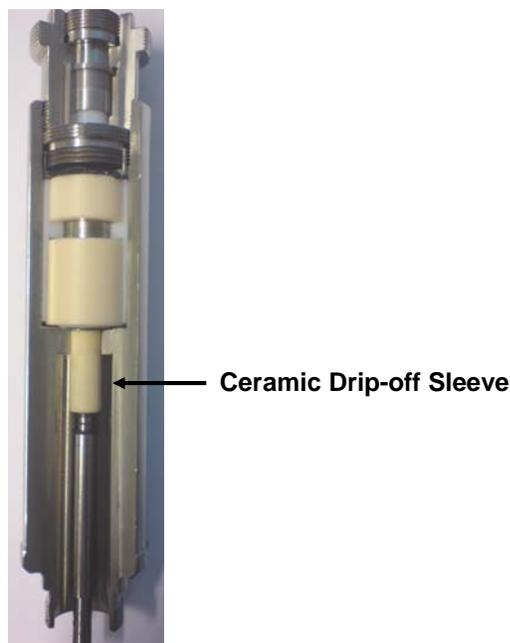
**Figure 3. High Pressure and High Temperature Seal Design.**
