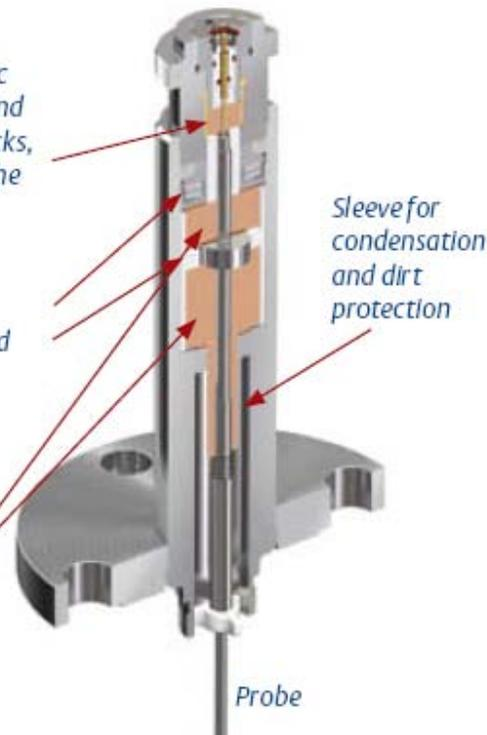
**Figure 2. Extreme pressure and temperature seal design.**
