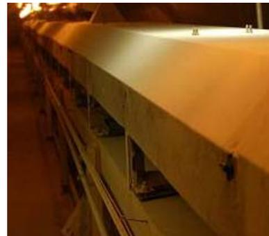
Each of the nine conveyor belts had four bearing temperature measurements and four rub block temperature measurements that were handled by one 848T FOUNDATION™ Fieldbus High Density Temperature Transmitter.
