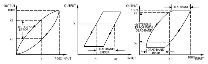
For control valves, dead band is the dominant nonlinearity whereas hysteresis is a secondary effect. Hysteresis can be estimated by subtracting dead band from the dead band plus hysteresis data. However, since hysteresis is generally negligable and difficult to discern from experimental error, dead band and hysteresis are not separated and test results are reported as the sum of these nonlinearities.
