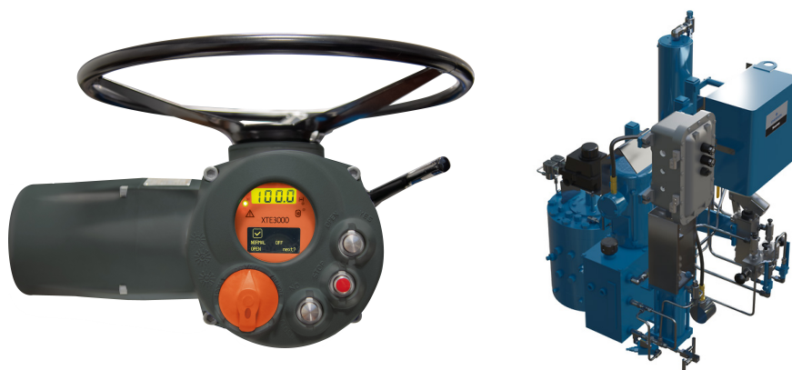
Figure 12: When air is not available, advanced electric actuators with or without spring fail assist are available (Bettis™ XTE top). For high torque applications, zero emission options, like the Shafer™ ECAT SHO (bottom), use pipeline gas pressure to drive actuator hydraulics.
