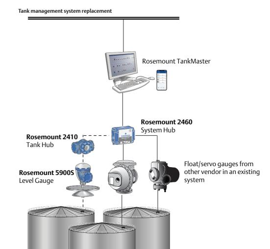
Replacing old tank monitoring software with TankMaster.
