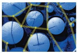
Figure 9.7: A self-organizing mesh field network can automatically find the best way around any fixed or temporary obstacles.
