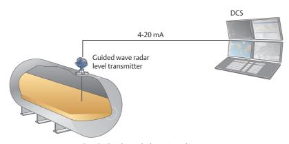
Figure 5.4: Typical process level transmitter architecture.
