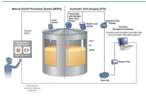
Figure 10.8: The traditional (obsolete) approach to overfill prevention - manual systems based on point-level measurement.
