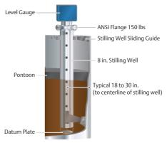
Figure 3.3: Still-pipe attached to the tank wall.
