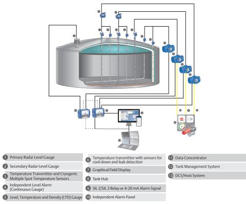
Figure 7.5: Example of a high performance full containment tank gauging system.
