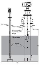
Figure 2.7: Servo gauge and temperature sensor measuring inside
