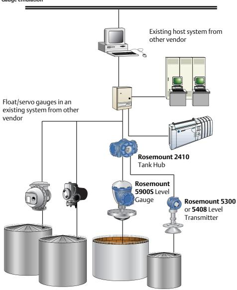
A Rosemount device can seamlessly replace a gauge from other vendor, independent of measurement technology. Data from the tank is displayed as before on the existing inventory management system.
