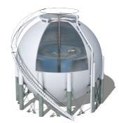
Figure 4.3: A pressurized tank with product in both liquid phase and gas
