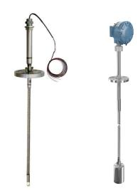
Figure 6.2: Left - Multi-spot temperature sensor with Pt100 elements and corrosion resistant metallic sheath. Right - Complete temperature measuring assembly with transmitter, sensor, optional water level sensor and anchor weight.
