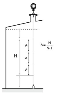
Figure 6.3: Spot temperature elements should be placed with equal distance between each element.
