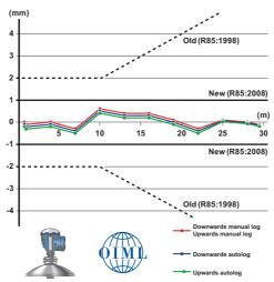
Figure 5.1: Graph showing OIML level accuracy requirements with a high performance radar gauge.
