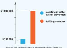
Figure 10.4: Comparison of two investment options that both correspond to an increase in volume equivalent to one tank.
