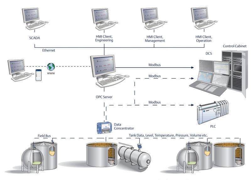
Figure 9.1: Modern tank gauging system architecture.
