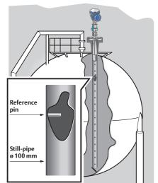
Figure 7.1: Level measurement in a spherical gas tank using a still-pipe with reference pins.
