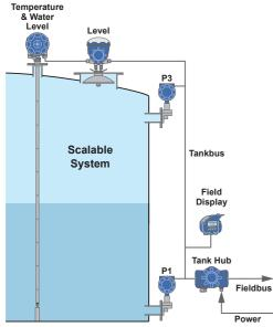
Figure 9.2: Intrisically safe field bus providing power and communication to
