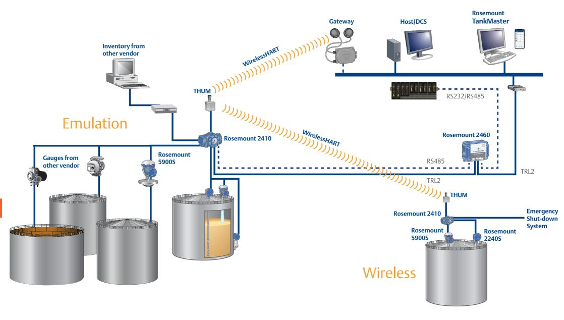
Adding a wireless network can bridge the gaps of the legacy bus system. By doing this, the user can get an additional communication channel for gauging, configuration and diagnostics.
