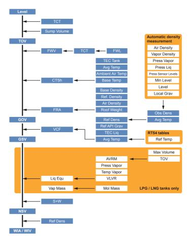
Figure 4.4: Detailed volume calculation flowchart.
