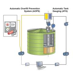
Figure 10.11: System overview for 2-in-1 radar level measurement.
