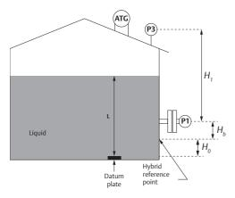
Figure 8.1: Density measurement is carried out with the help of a level gauge and one or two pressure sensors.
