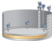
Figure 1.8: Up to six guided wave level transmitters can be installed directly on the floating roof, with rigid probes penetrating through the roof and into the liquid below. Roof till is tracked by comparing the distance from the floating roof down to the product surface. With one or two extra transmitters one can also detect if the roof drain gets plugged or if there is any hydrocarbon on the tank roof.
