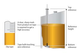
Figure 2.4: Manual level measurement definitions.
