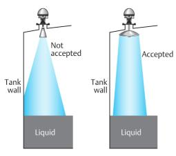
Figure 2.15: Radar gauges with wide beam (small antenna) and narrow beam (large antenna).
