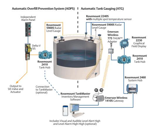
Example of a modern approach to overfill prevention, incorporating an automatic overfill prevention system based on continuous radar level measurement.
