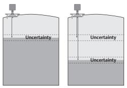
Figure 5.2: Uncertainty when measuring batches could be reduced by offset error elimination.
