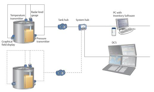
Figure 5.5: Typical tank gauging system architecture.
