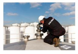
Figure 2.2: Hand gauging with a dipping tape.
