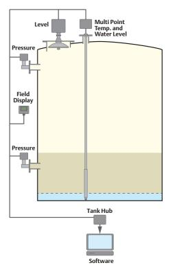
Figure 3.6: Hybrid tank gauging is a combination of a traditional tank gauging system and an HTG system.
