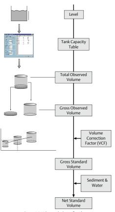
Figure 4.1: Volume calculation flowchart.
