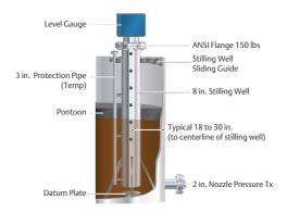
Figure 3.2: Still-pipe attached to the tank bottom.
