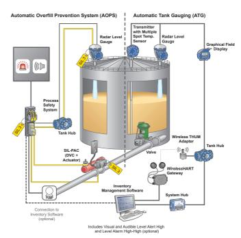
Figure 10.9: Example of a modern approach incorporating an automatic overfill prevention system based on continuous radar level measurement.
