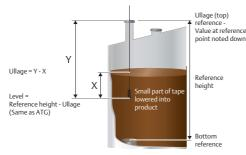
Figure 2.3: Manual ullage measurement definitions.
