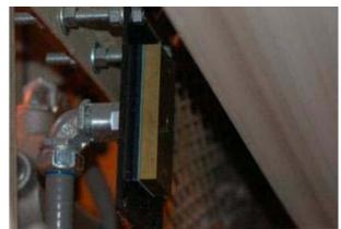
Rub blocks provide an indication when the conveyor is even slightly out of alignment. A conveyor out of alignment can be a potential ignition source.
