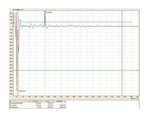
Figure 2. During start-up, the Emerson technician took an echo plot to confirm surface level and saved it for future reference.
