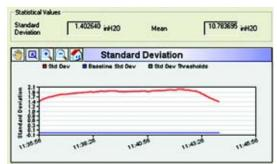
The amplitude of the process noise, indicated by Standard Deviation (red line), shows the presence of pulsation. If no pulsation were to exist, the process noise would be closer to the baseline (blue line).
