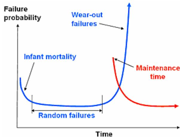
The cycle starts with a high probability of premature (infant) failures that result from manufacturing or installation errors. The probability of failures is then relatively level until the equipment begins to wear out. Preventive maintenance is scheduled to take place before this probability increases significantly.
