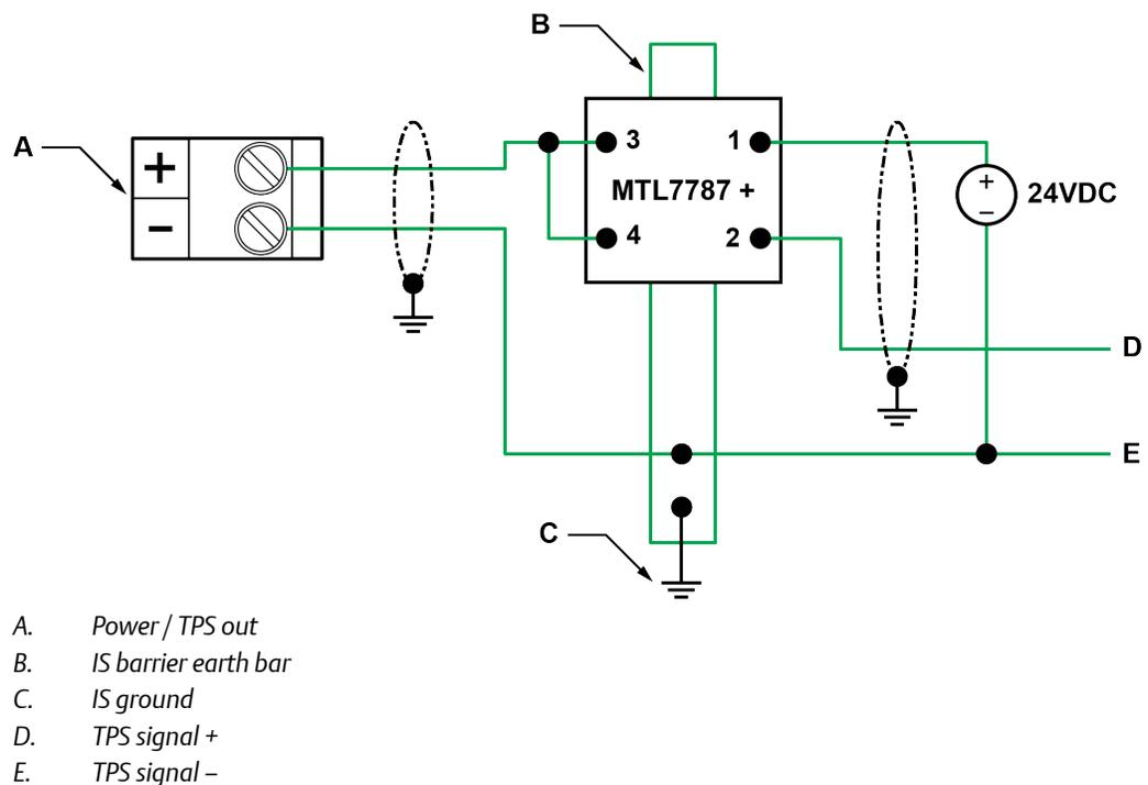
Figure 3-4: 2-wire barrier connection plus RTD barrier connection
