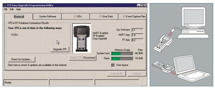
Easy Upgrade allows communication between the 375 Field Communicator and a PC using IrDA. The IrDA port enables transfer of configuration data between the 375 and AMS Device Manager as well as upgrading of new Device Descriptions and functionality.
