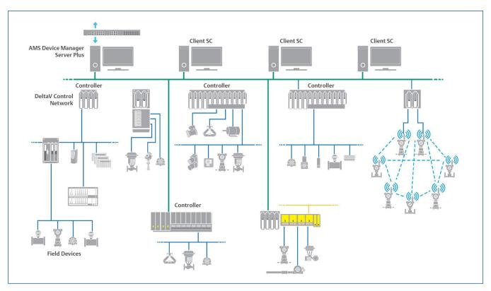
Using AMS Device Manager with the DeltaV system enables you to access important HART, FOUNDATION Fieldbus, WirelessHART, PROFIBUS PA, and PROFIBUS DP device data with no additional cabling or field wiring required!
