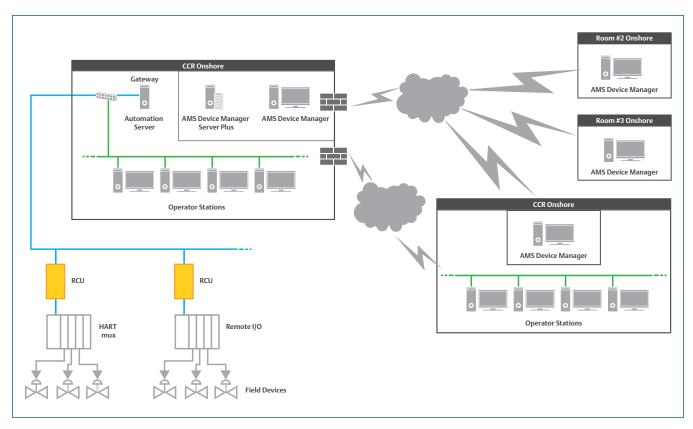
Gain online connectivity to HART devices in offshore oil and gas applications with AMS Device Manager and the Kongsberg Maritime system.
