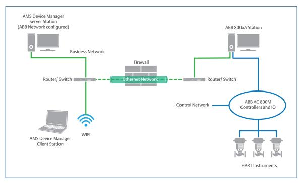
This example architecture shows how AMS Device Manager can be deployed with ABB System 800xA.
