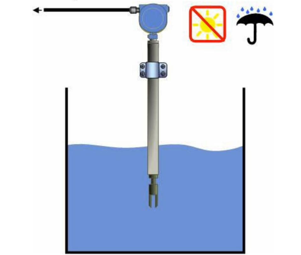
2. Confirm the meter tines are away from the tank wall.
