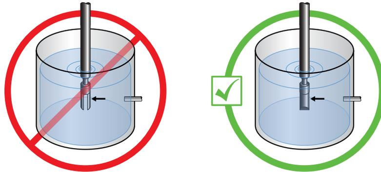
8. Confirm the meter tines are kept away from deposit buildup.
