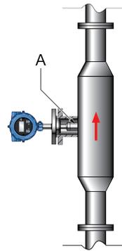
A. FDM directly inserted into the flow
