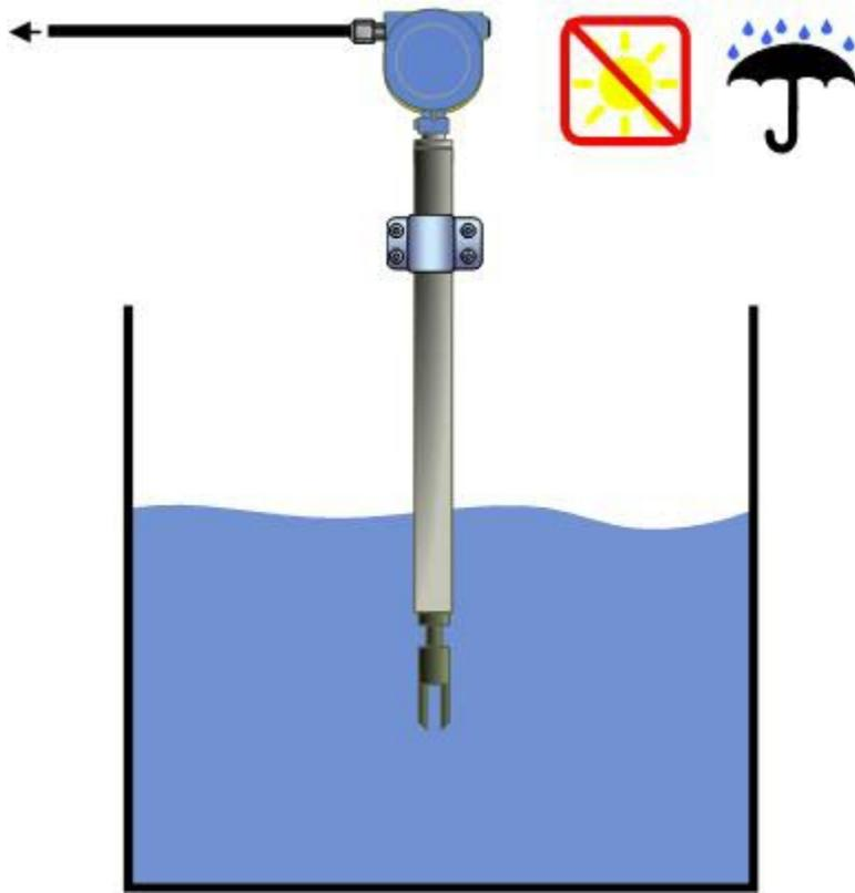
2. Confirm the meter tines are away from the tank wall.
