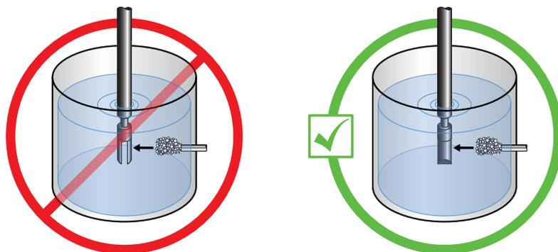
6. Confirm the meter tines are kept away from deposit buildup.
