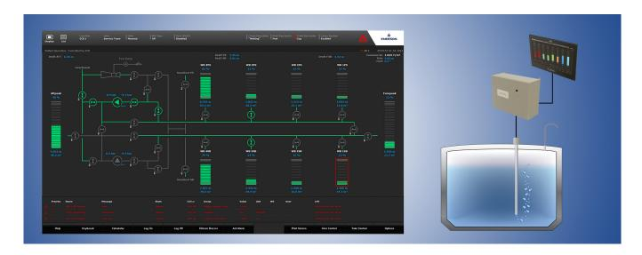
The electro-pneumatic tank level gauging system provides reliable information on tank levels, tank volumes and ship's draft. The system provides solutions for all types of vessels measuring ballast, fuel, miscellaneous tank and void spaces using electro-pneumatic technology. The system offers trouble-free ownership with limited life-cycle cost, ease-of-use configuration and fault finding utilities.
