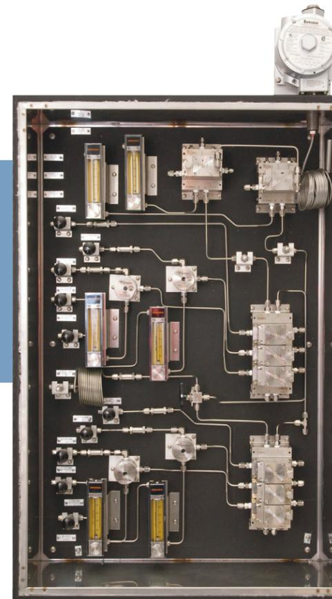
Emerson custom-engineers sample systems to meet the specifications of each unique requirement. Common features include heated and open panel designs, automatic calibration/validation, and a variety of sample probes to extract a reliable and stable sample from the process. In addition, sample systems and all related components can be rated for area classification.
