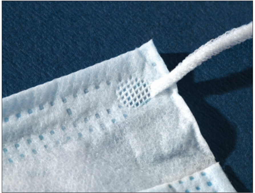
Ultrasonic welds strongly bond even small items like the ties on a disposable surgical mask at a fraction of the cost of stitchery or glue and can be used immediately. (Credit: Emerson)
