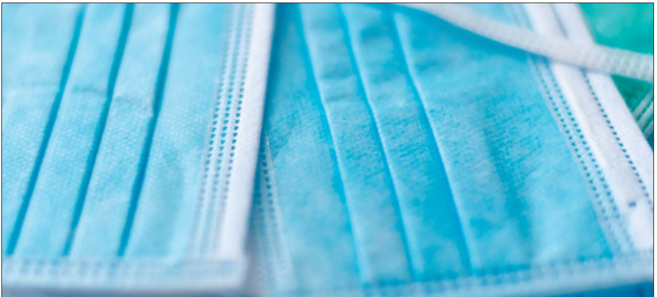
Medical mask production utilizes continuous ultrasonic welds for seams on the width and length of the mask, while the tie straps or elastic ear loops are bonded with plunge or "spot" welds. (Credit: Emerson)
