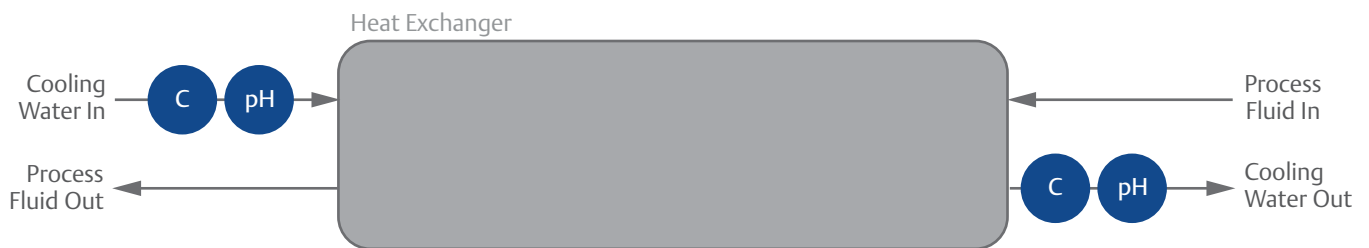
Figure 1 - Heat Exchanger Leak Detection Process
