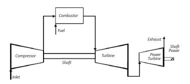
Stoichiometric combustion is the ideal combustion condition where fuel is burned completely. Complete combustion is a process burning all the carbon (C) to (CO $_2$ ), all the hydrogen (H) to (H $_2$ O) and all the sulfur (S) to (SO $_2$ ). Almost all modern turbines require stoichiometric combustion. Any unburned components remaining in the exhaust gas, such as C, H $_2$ , and CO, means the combustion process is incomplete and not stoichiometric.
