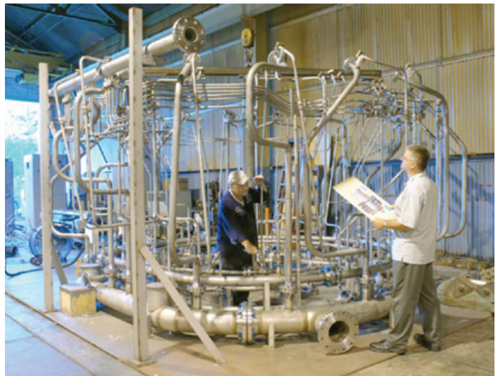
6. Interferences required changes to standard engine injection-water and fuel piping (left). Engineer responsible for the redesign effort was at the factory during fabrication (right)
