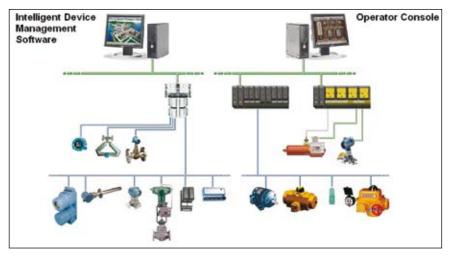
The position of device management software in the automation hierarchy. (Handheld communicators can also be used to access devices).
