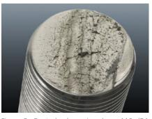
Figure 2. Control valve noise above 110 dBA external to the pipe can fatigue bolts and ultimately crack control valve stems and shafts. For this reason, sound levels should be kept below this threshold.
