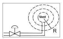
Figure 1A. Noise point sources lose sound energy quickly, falling with distance squared.
