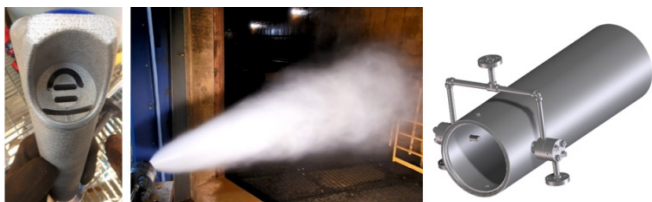
FIGURE 6: High pressure steam is injected at the flow nozzle (left) to completely atomize the water under a wide variety of water flows and process pressures (middle). The steam-atomized atomizer (right) was specifically designed as a retrofit to the existing spring-loaded nozzle atomizer to minimize piping change
