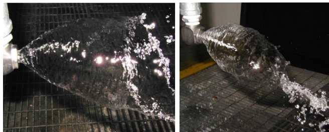
FIGURE 3C (left): As nozzle pressure drop continues to fall, the spray turns to a sheet of water. Eventually the falling pressure drop will result in water simply pouring into the pipe as shown in FIGURE 3D (right).
