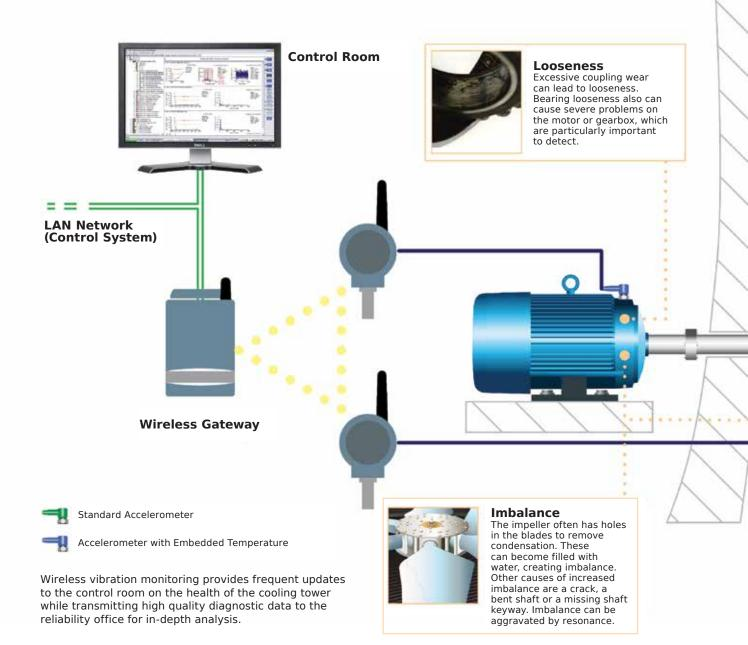
ance caused by damage to one of the fan blades. Misalignment of the long shaft between the motor and gearbox, referred to as the jackshaft, also can lead to excessive coupling wear. However, the most common culprit is the gearbox itself, which can suffer from broken, chipped or worn gear teeth as well as defects in the bearings. These issues frequently find their root cause in insufficient lubrication.
