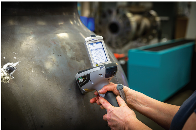
FIG. 2. While a PMI gun can reveal some details regarding materials of construction, it does not provide a complete picture. Source: Emerson.
