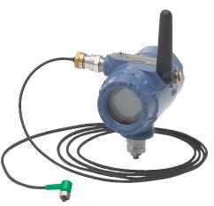
**Figure 1**. An Emerson CSI 9420 Wireless Vibration Transmitter sends equipment data to an integrated plant control network via a wireless gateway. According to one refiner, these field devices can typically be installed in a couple of hours compared with a couple of days for a wired device.
