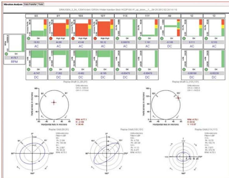
**The transient data facility enables simultaneous monitoring and recording of multiple channels – the system records up to 100 hours onto a hard disk, which can be replayed should an event occur (illustrations: Emerson Process Management)**
