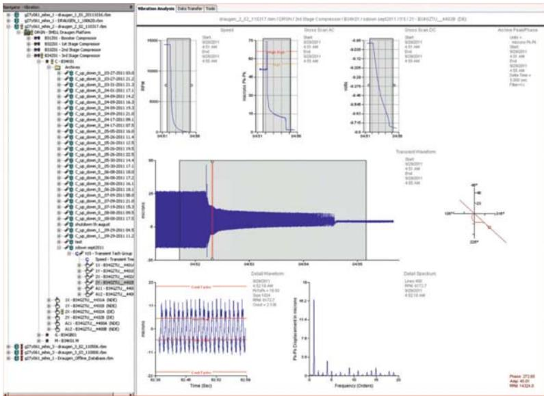
**Using the transient data facility in AMS Machinery Manager, operators were able to quickly identify the heavy spot to enable rebalancing**
