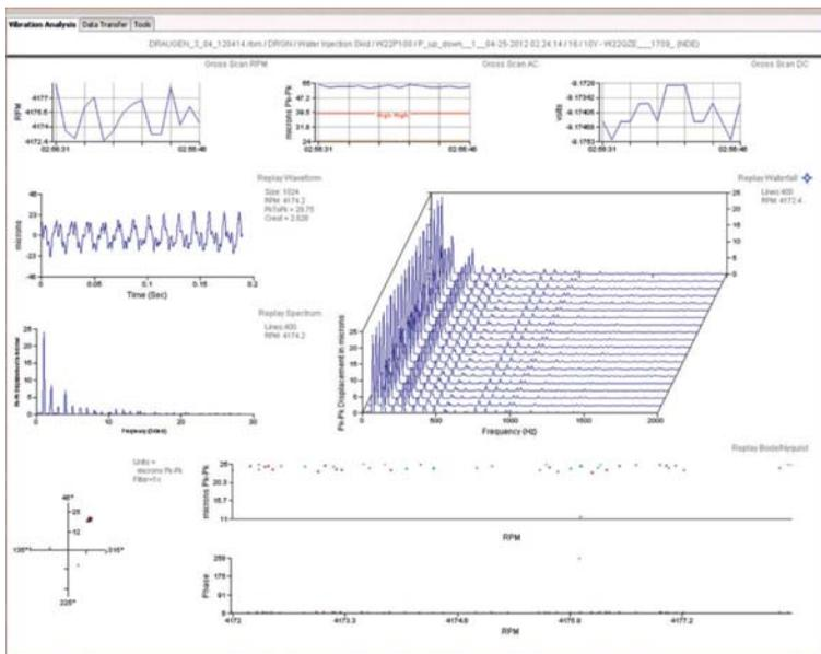
**The live mode in AMS Machinery Manager provides real-time data plots, including overall levels, orbits, shaft centre line, Bode/Nyquist, cascade, waveform and spectrum**
