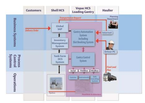
**Schematic of Shell Pernis loading operations**
