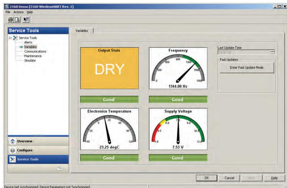
*Device details such as frequency and power module status facilitate troubleshooting.*
