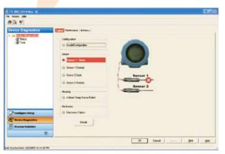
Temperature transmitter diagnostics indicate sensor failure.
