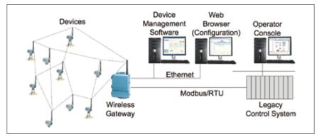
A wireless gateway enables legacy control systems to receive process variables from wireless transmitters.
