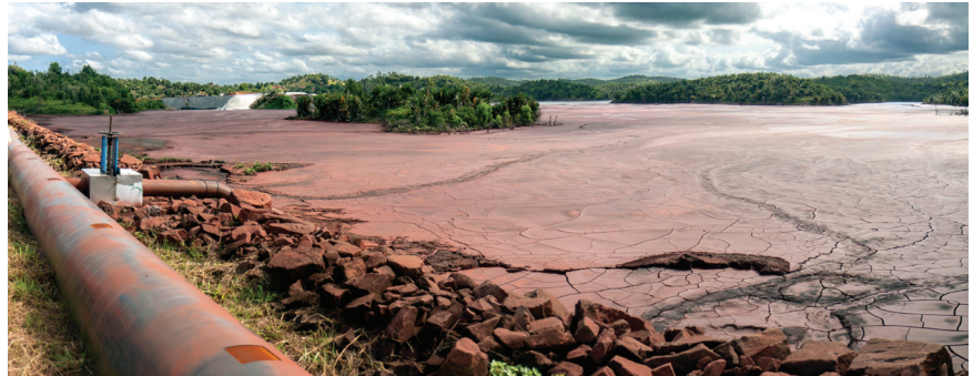
Figure 1: Increased water recovery efforts are creating tailings slurries that are far denser and more abrasive.
