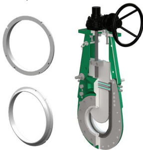
Figure 3: Hardened wear rings on both sides of the valve body absorb the bulk of the slurry impact and protect the valve components. These rings can be rotated, and the valve body can be reversed to extend service life. (Pictured here is Emerson's Clarkson KS3 Severe Service Knife Gate Valve.)
