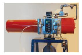
components that include a sensor, logic solver and final element (FE) – actuator, controls, pressure relief components and quarter-turn valve performing a Safety Instrumented Function (SIF). To ensure system reliability, industry standards, most notably IEC 61508 and 61511, have been implemented to manage the veracity of the system.
