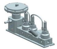
This assembly, which consists of an air-actuated regulator with a pressure transducer and isolation valves, provides automated pressure regulation while reducing the installation footprint and leak paths for critical aerospace applications.
