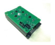
**Absolute Position Detector** provides precise valve position under all conditions including loss of power, no battery backup required.
