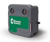
Pneumatic Controllers are mechanical devices designed to measure temperature or pressure and transmit a corrective air signal to the final control element. Boundon tubes, bellows, temperature elements, or displacers are used as the sensing elements. The power supply and output of a pneumatic controller is compressed air or natural gas.  $\blacktriangleright$  4194 | 4195K | 4196 | 4660 | C1
