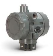
Electro-Pneumatic (I/P) Transducers convert an electronic signal to a pneumatic signal. They are routinely used in control loops that require an electronic control signal from a programmable logic controller or distributed control system to be converted to a usable pneumatic signal for operation of a control valve. ▶ 646 | 846 | i2P-100
