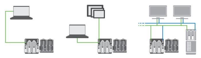
Operate and configure your standalone applications with PK Controller Engineering software and PK Controller Engineering Station. Standalone PK Controllers do not require a permanent connection to a ProPlus to operate, PK Controller Engineering Stations provide a temporary local connection. For increased availability, get easy redundancy by simply installing the redundant controller onto the carrier next to the primary – with no added cabinet space or configuration change.
