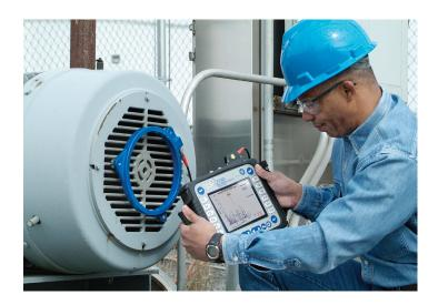
Flux measurements should be taken monthly to measure any deviation of the electromagnetic field. Generally speaking, while rotor defects on AC motors progress slowly, stator faults can develop rapidly. Therefore ,frequent monitoring is recommended.
