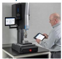
Adjustable down speed control with energy and force profiling during a weld are key benefits of the electro-mechanical advanced actuation technology
