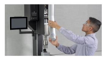
Electro-mechanical advanced actuation system, available with the Branson GSX-Elite precision series, instantaneously adjusts based on real-time feedback. This improves accuracy across a wide range of applications and components (closed loop).
