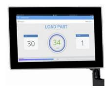
Intuitive HMI with touchscreen display located directly in operator's line of sight ensures operators always have access to critical, actionable weld data.
