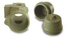
The XL Commando range solves aggressive corrosion problems. It works where stainless doesn't. A proprietary heat treatment with CG941 fluorpolymer impregnates the body making it impervious to corrosion. The steel pinion is also fluorpolymer coated. Field service has shown that the Commando actuators outperform other actuators in corrosive environments.
