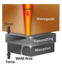
Laser emitting waveguides can be configured in 3D to conform exactly to the geometry of the part surfaces they are to join, melting the entire surface interface at once for a fast, uniform weld joint with precise melt collapse control.
