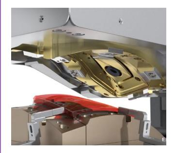
Laser welding puts no mechanical stress on parts, therefore there may be no need for annealing, or less annealing time required, to relieve internal material stresses.
