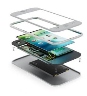
Electronics and sensitive components can be embedded in welded parts.
