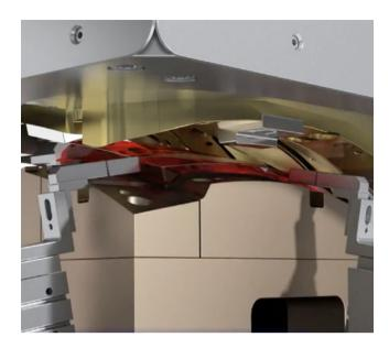
With no movement of the parts during joining, this leads to a more precise weld and hermetic seals can be created if required.
