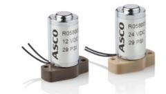
Direct acting solenoid valves for use with neutral or aggressive liquids, with special media separating soft-seal PTFE diaphragm preventing any potential leakage of critical reagents within the instruments compartment.
