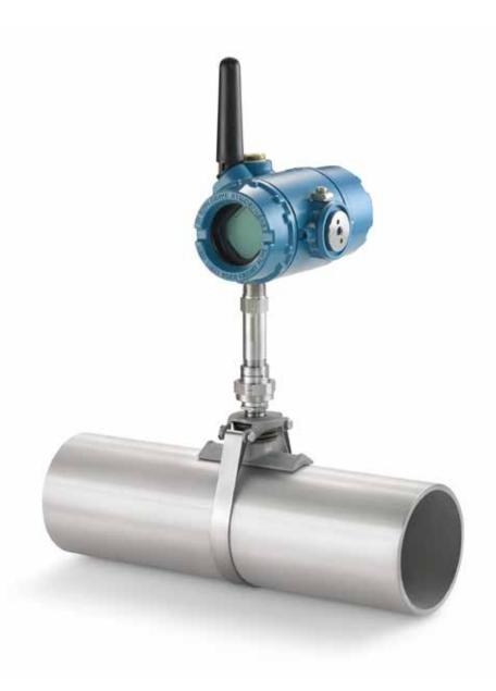
Rosemount X-well Technology uses an algorithm based on Fournier's Law that incorporates surface temperature, ambient temperature, and pipe characteristics. This allows Rosemount X-well Technology to calculate and output process temperature with similar accuracy to a traditional insertion thermowell and sensor configuration.
