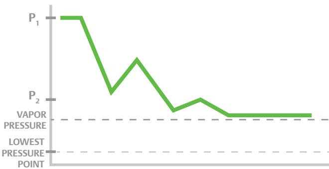
**Cavitation Prevention** is possible as the liquid undergoes a portion of the total pressure drop in each stage. This prevents the liquid in any stage from falling to or below its vapor pressure, avoiding cavitation.
