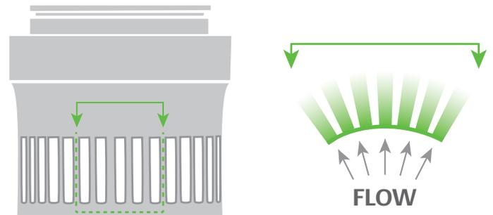
**Exit Jet Independence** is crucial for avoiding jet coalescence, which will lead to additional noise. All Emerson noise technologies are designed with this critical factor as standard.
