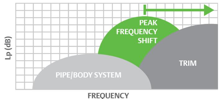
**Frequency Spectrum Shifting** reduces strain and acoustic energy in piping by exploiting the natural damping of high frequency acoustic waves. Piping transmission loss is maximized to reduce radiated aerodynamic noise.
