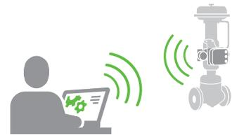
**Valve Connected Services** are a part of the Plantweb™ digital ecosystem and provide the ability to gather and aggregate diagnostic data across a single site and multiple sites across the globe. Emerson's certified analysts will interpret positioner data to look for patterns of systemic degradation and provide recommended actions to minimize downtime.
