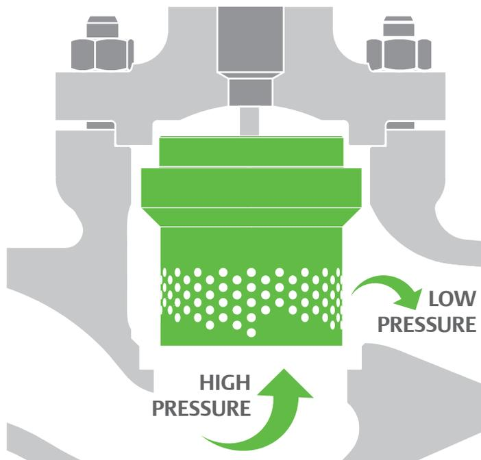
**Pressure Management** utilizes the expanding area principle to allow for volumetric expansion of depressurizing gas and safe pressure reduction of potentially cavitation liquids.
