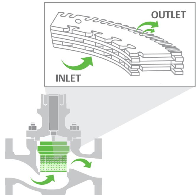
**Unique Flow Passage Shapes** reduce turbulence to minimize shock-associated noise and place turbulent shear layers away from solid boundaries to reduce noise. The multi-stage pressure reduction, utilized with sound engineering principles, controls jet size, formation, interaction, and accommodates fluid expansion.
