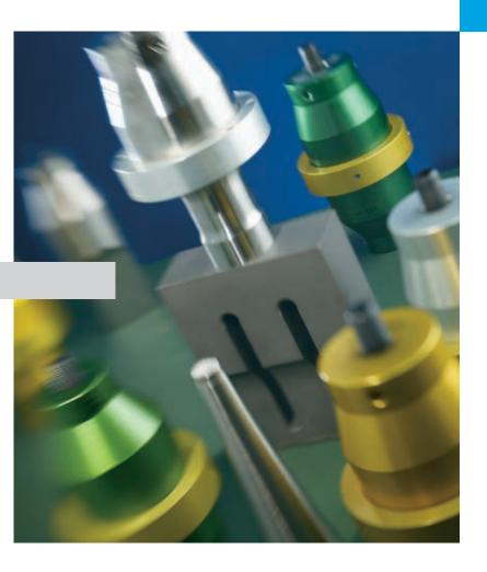
Ultrasonic welding is well suited for assembling parts with delicate internal electronic components and can be used to insert, stake, stud weld, degate, or spot weld thermoplastics, and slit or laminate thermoplastic films and fabrics.
